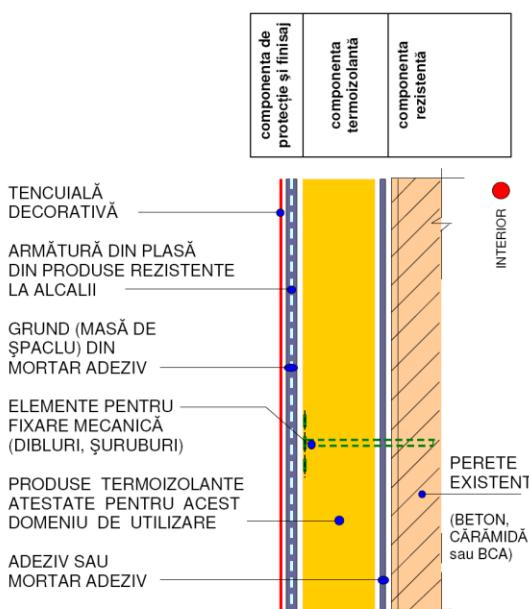
**FIGURA 2 – SISTEM TERMOIZOLANT CU STRAT DE AER VENTILAT**
