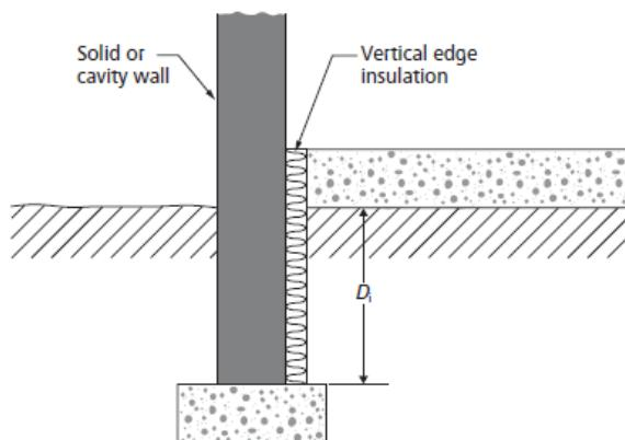
Figure 3.11 Solid ground floor with vertical edge insulation
