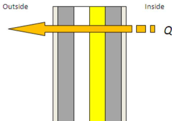
**Thermal Transmittance through multilayer element**
