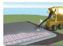
8 Insulated foundation system is now complete and ready to take 100mm concrete.
