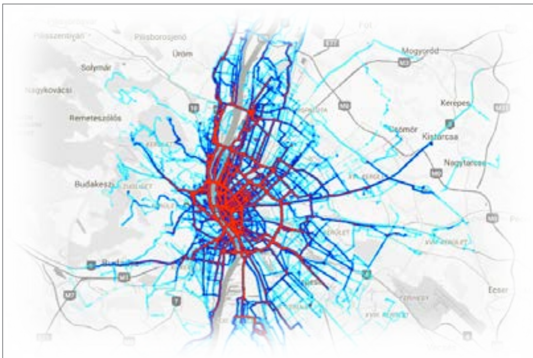
Figure 5: Macroscopic modelling for the city of Budapest. Source: FLOW project
